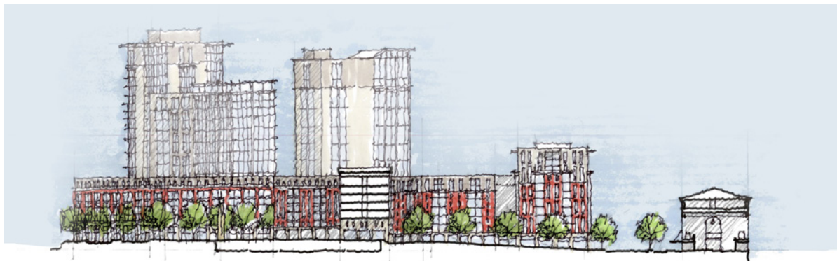
Section through the site, looking north, Union Station to the right. The change in grade from one side of the site to another provides the ability to insert a level of parking under the buildings without it being visible on the perimeter of the site,
