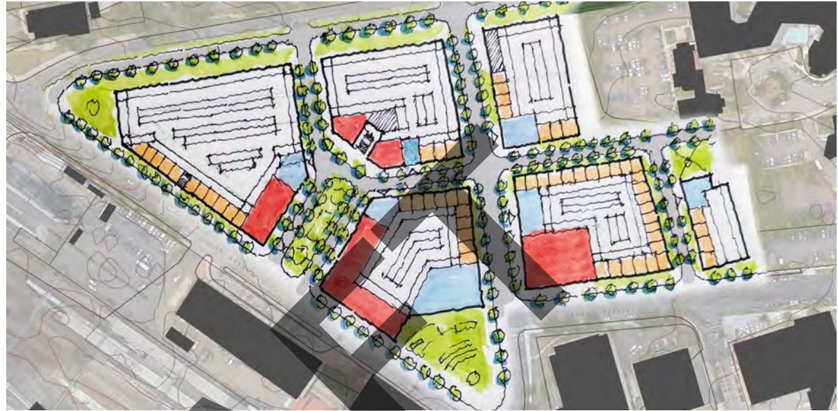
Figure 57: Ground Floor Plan showing parking lined with retail (red) and amenity (blue). The parking along Church Street S is buried underground and is not visible from the street
